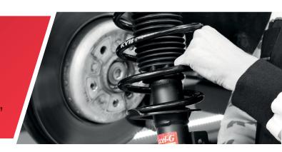
Noticing fluid on the outside of a shock absorber or strut doesn't necessarily mean that the product is leaking. A true leak signals a loss of vital fluid and can quickly lead to reduced ride control and safety issues. In contrast, "sweating" is often the result of normal operation as the seals lubricate themselves. Knowing the difference can save you from unnecessary repairs:
