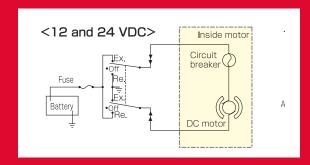
Use a bipolar, double throw, instantaneouscontact type switch with the switching off position at the neutral point at the center for 12/24 VDC switching.
