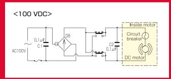
Use a 100-VDC MMP with the 100-VAC power supply via a full-wave rectifier.
