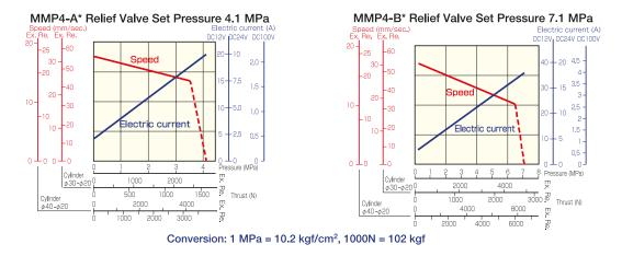
The above charts show the characteristics of MMP without the slow return valve orifice [ (9)]. Cylinder extension and retraction speeds differ due to the receiving area difference.
