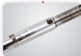
Damaged piston rod
