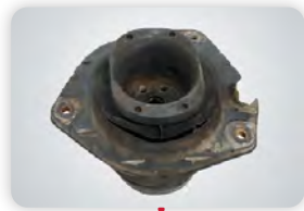
Torn Strut Insulator
