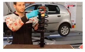
If the top plate is not positioned correctly, the spring will bend. This will make a noise and may even touch the inner wing.
