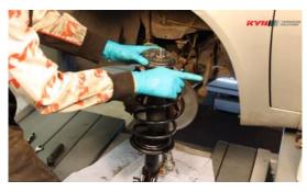
The strut mount is on the bearing which can rotate to have the strut assembly fitting the car body correctly. The strut mount must be positioned at a 90 degree angle from the top plate slot. It's important that the strut mount is facing in the right direction, as per these photos.
