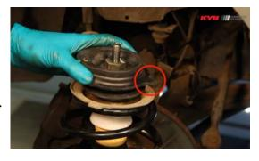
KYB has a fitting video on YouTube to help explain the correct alignment and fitment of this Fiat Punto front coil spring.
