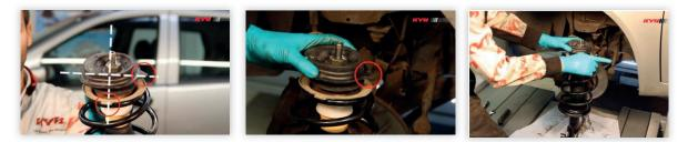
The strut mount is on the bearing which can rotate to have the strut assembly fitting to the car body correctly. The strut mount must be positioned at a 90 degree angle from the top plate slot. It's important that the strut mount is facing in the right direction, as per these photos.
