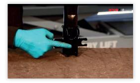
The top plate slot must be in line with the lower knuckle bracket of the shock absorber.
