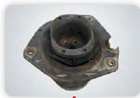
Torn Strut Insulator
